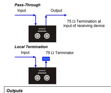
Slave output streams can be connected or disconnected without disturbing the source bitstream.
